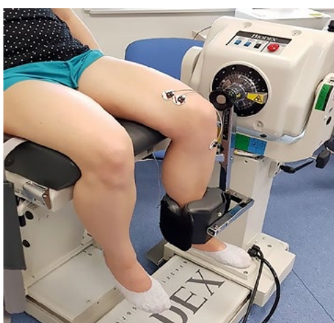
Figure 3. Position of the lower limb of the participant in flexion of the knee joint at the angle of 90° during the sEMG test with the use of the BIODEX system – position No. 2.
